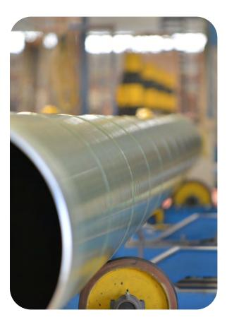
• Dual layer abrasion resistant over OD coating FBE+ARO (ARO): API 5L7, CSA Z 245-20, NACE RP 0394,
